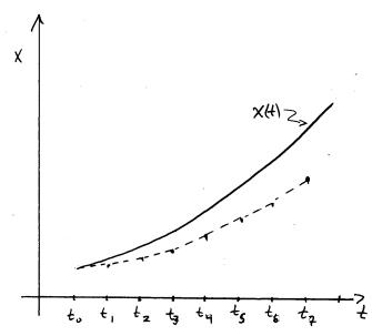
The deviation from the exact x(t) may tend to increase as the total truncation error accumulates from step to step, the further we get from the initial values  $(t_o, x_o)$ . The lesson is—make *h* small.
