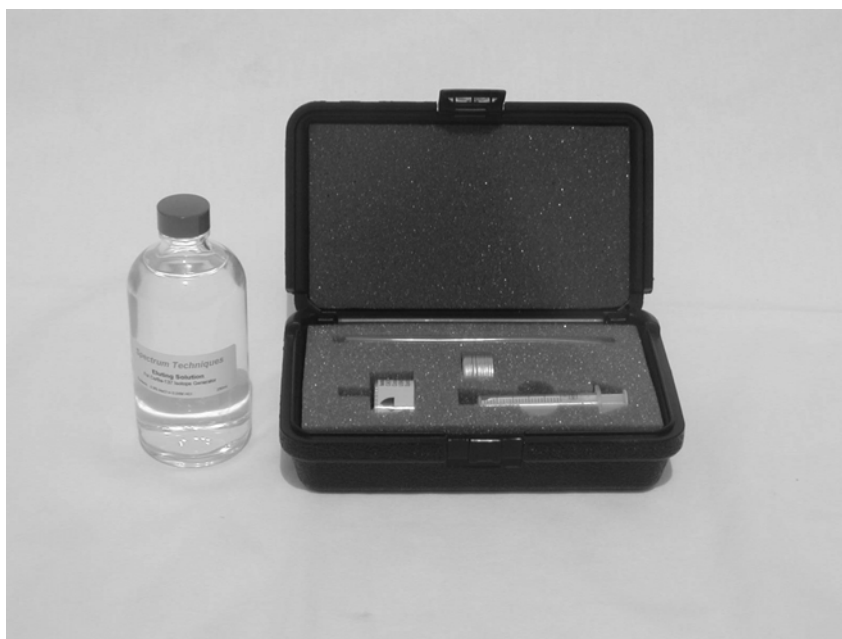
Figure 3: Isotope Generator to make Ba-137m from Cs-137
