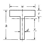
Use the function to determine  $y_c$  for an area with w = 240 mm, h = 380 mm, d = 42 mm, and t = 60 mm.
